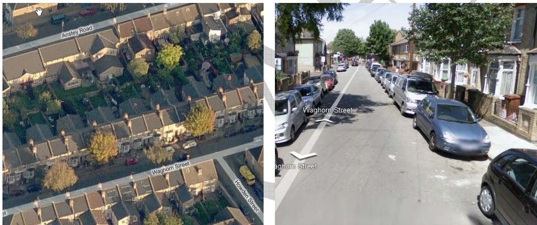
Block 13 Waghorn Street. 2 – 3 storey terrace housing. Approximately 97 dwellings per hectare. Small building setbacks (1.5 metres) with few street trees along narrow footpaths. Private gardens small (approximately 60sq.m)
