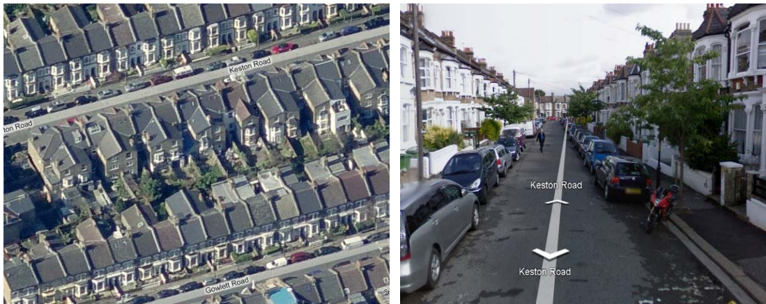
Block 12 Keston Road. 2 – 3 storey terrace housing. Approximately 114 dwellings per hectare. Small building setbacks (2.5 metres) with few street trees along narrow footpaths. Private gardens small (approximately 50sq.m)
