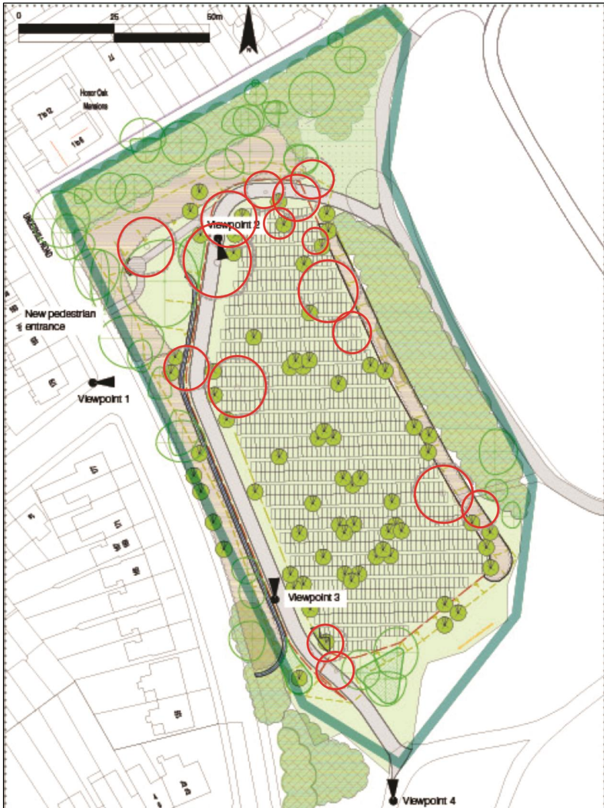
Plan 4: Original works plan provided for the Preliminary Bat Assessment, showing trees to be removed.
