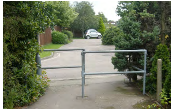
Fig. 1.36 - Typical entrance/exit chicane
