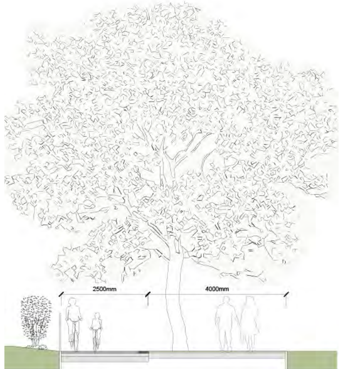
Fig. 1.99 - Quietway on extended self-binding gravel path
