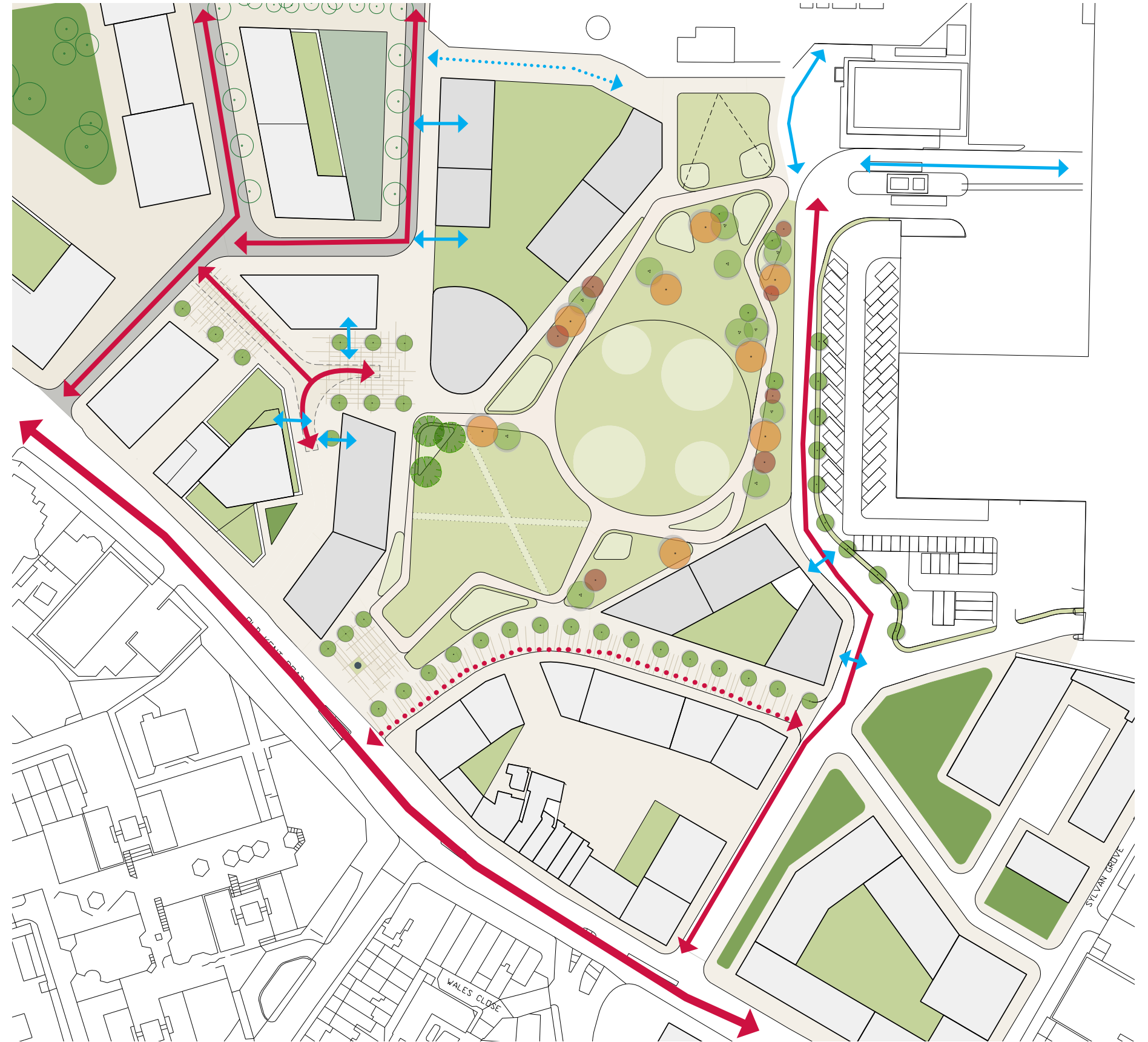
Figure 130: Alternative masterplan - Servicing diagram
