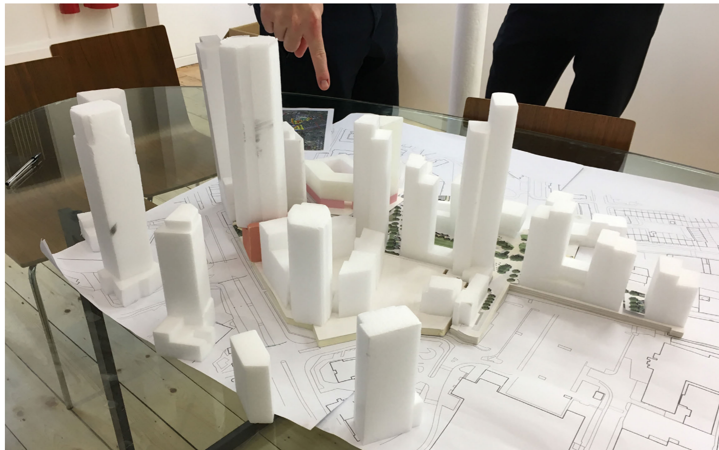
3D massing models were used to test the proposed towers where three Opportunity Sites intersect
