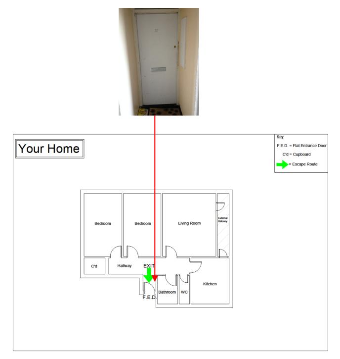
The plan above is a typical flat layout; however, your flat layout may vary slightly. If so, ensure you identify the various exits using the photos and plan and exit via your front door or the alternative means of escape doors.
