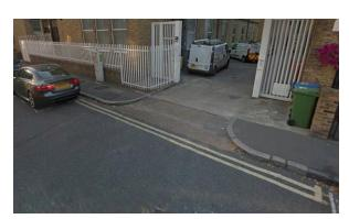
b. If a Vehicle Crossing is not located on a Classified Road then double yellow lines should be provided for the entire length of the Crossing plus ≥ 2m to either side.
