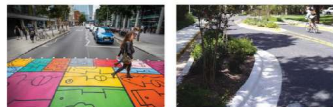
Traffic calming measure along Mandela Way could include raised crossings and planted chicanes through the park
