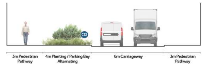
B - New Verney Road - Working Street Section
